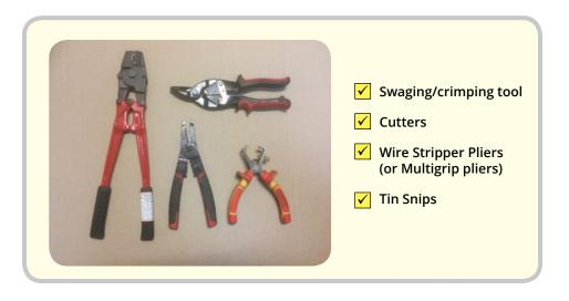
1 Remove plastic from the wire by cutting with snips along the inside of the bead. Then bend the centre panel up and out the way. Then using wire stripper pliers remove the polymer from the wire. The length of polymer to be removed should equal the length of the swage you are going to use. We have used a double swage here which is 22mm long. Smaller swages can be used in pairs to provide a sufficient join.
