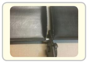
On our double swage crimp 3 times to provide suitable grip. Repeat the process on the other wire.
