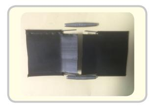
Insert the exposed lengths of wire into each end of the wire vise joiner as shown below. When completed there should be no exposed wire, and there should be a small overlap in the centre polymer panel so that no gap appears in the rail.
